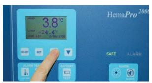
Check the temperature inside the storage unit, wait 30 minutes, without opening the door, to allow the temperature to stabilize and check it again to verify the thermostat should be adjusted.
