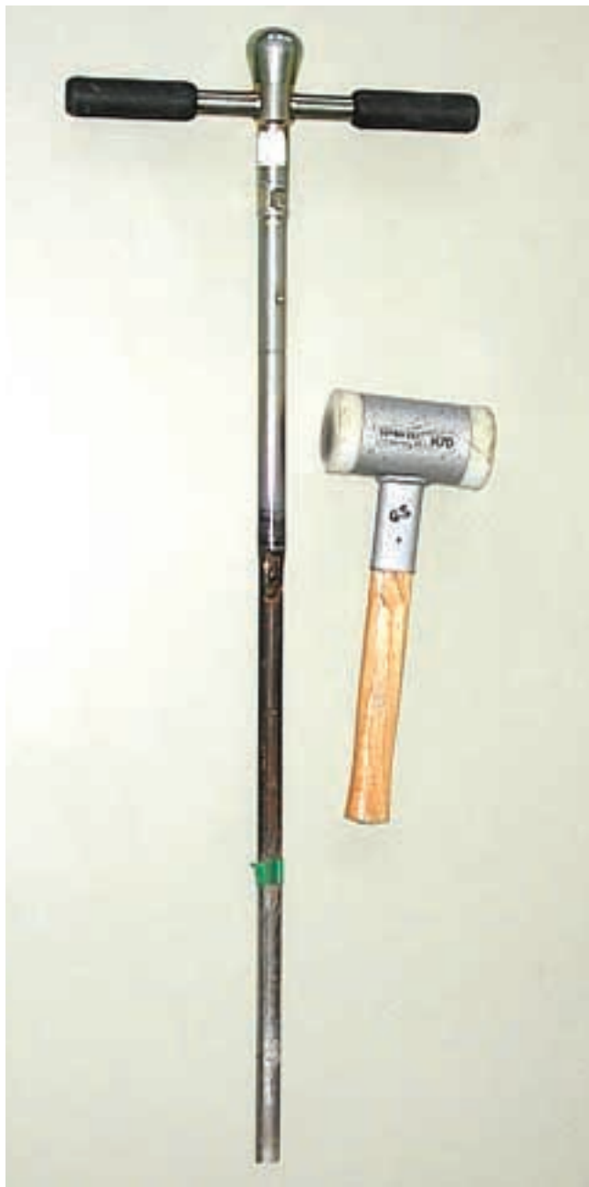
Sticker used for taking cores of soil.
