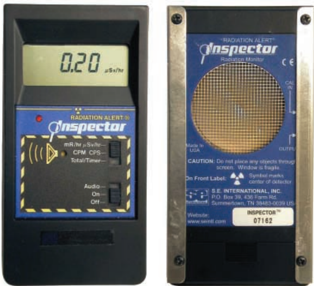
The Inspector instrument used for beta measurements, size 15x80x30 mm.
