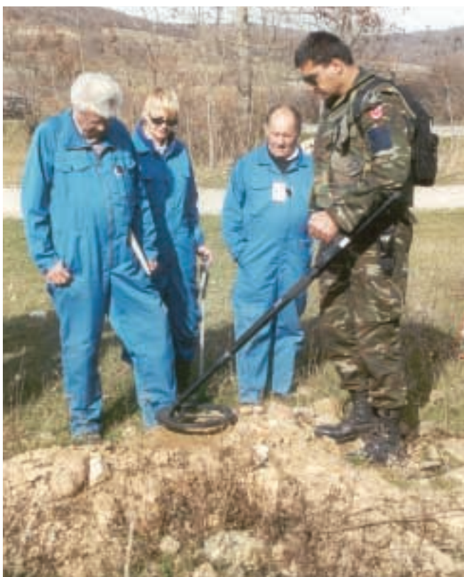
The Turkish EOD test their mine detector for its ability to find a DU penetrator.
